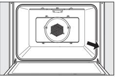
The silver data plate is located along the front side of the oven with the door open.
